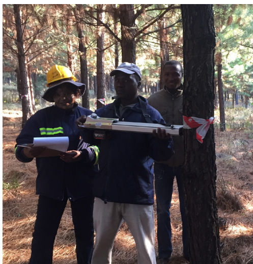
Safcol foresters Eunice Sehlabela (left), Daniel Khumalo and Clement Thabethe (right) take Resistograph readings in an 8-year-old pine hybrid trial in Brooklands, Mpumalanga, South Africa.
