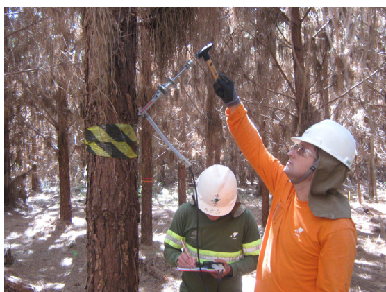
Ronaldo Donizete dos Santos (right) and Adalberto Custodio da Silva of Klabin take TreeSonic readings in a pine hybrid trial in Monte Alegre, Paraná, Brazil.
