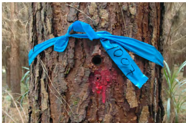
Figure 6. Care was taken to align extracted cores (upper hole) with Resistograph readings (small lower hole in the red paint). Both samples are bark to bark.
