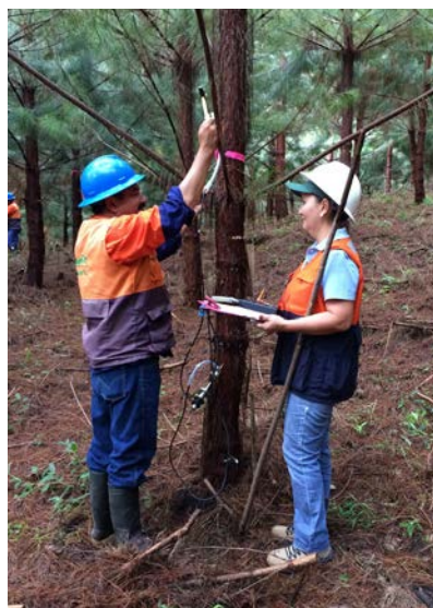
Ovidio Orrego and Liliana Perafán (SKC) using the TreeSonic to measure wood stiffness.
