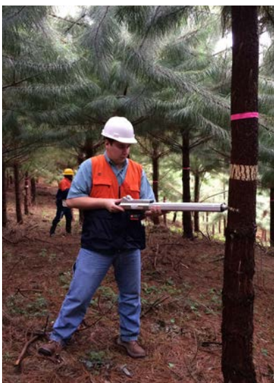
Juan José Acosta (Camcore) using the IML-Resistograph to measure wood density.
