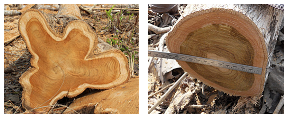
Measurements of internal and external diameters to assess heartwood percentage. Left is a buttlog, right is a more regularly shaped upper log.
