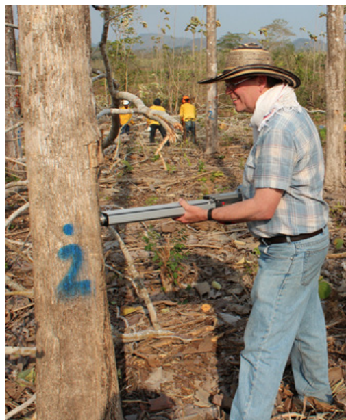
Juan López using the IML-Resistograph in a 16-year-old teak stand in Colombia to measure the density profile of the trees.
